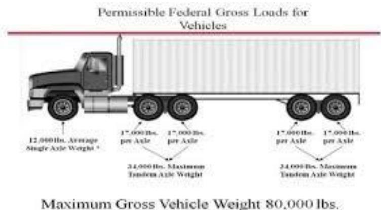
In addition to the Federal Gross Vehicle Weight Limit of 80,000 pounds for tractor/chassis/container gross weight, there is also a **weight distribution requirement, which states axle maximums of 12,000 lbs. – Steers; 34,000 lbs. – Drives; and 34,000 lbs. - Trailer/Chassis.**
